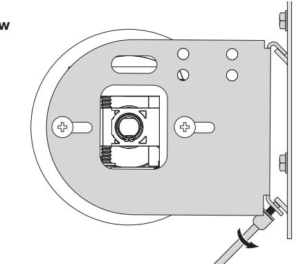
**CAUTION: RISK OF FALLING OBJECTS.** The shade bracket securing screw is factory-installed in the shade bracket, and must be tightened firmly into the sub-bracket to ensure safe installation of the shade. If the securing screw is missing, **DO NOT** substitute a different type of screw or omit Step d. Check the hardware kit for spare shade bracket securing screws, or contact Lutron for replacement screws. Failure to follow these instructions could result in minor to moderate injury.
